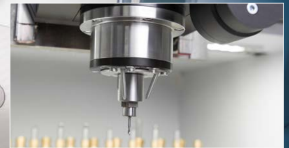
2 kW spindle and minimum-quantity coolant system
