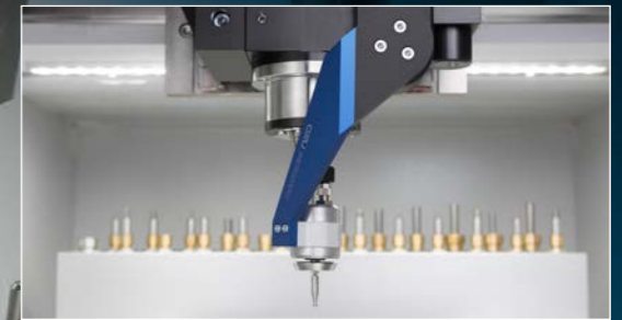
3D probe (XYZ sensor) and camera
