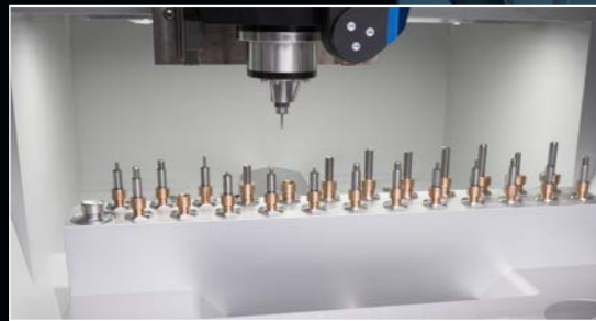
24-station tool magazine with integrated tool-length sensor
