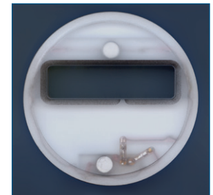
Step 2: Parts are secured with the vacuum fixture so that all of the detailed features that appear on the back can be machined.
