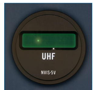
Photo 3: Black and white layers of paint are milled away on the top wall of the window opening.
