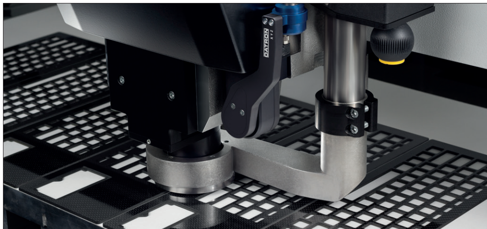
DATRON M8Cube high-speed milling machine initially researched by Carbide Products for machining aluminum parts.
