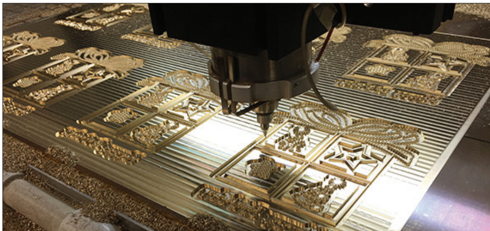
DC Graphics' ability to batch machine brass embossing dies results in high efficiency and short lead times for their customers.
