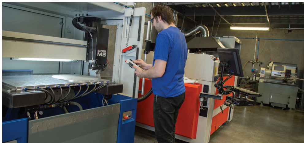
Lead machinist, Ilya Pasumanskiy, positioning the spindle of the DATRON machine using its hand-held remote.
