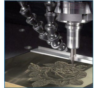
Hallmark embossing die engraved on DATRON M8 high-speed CNC.
