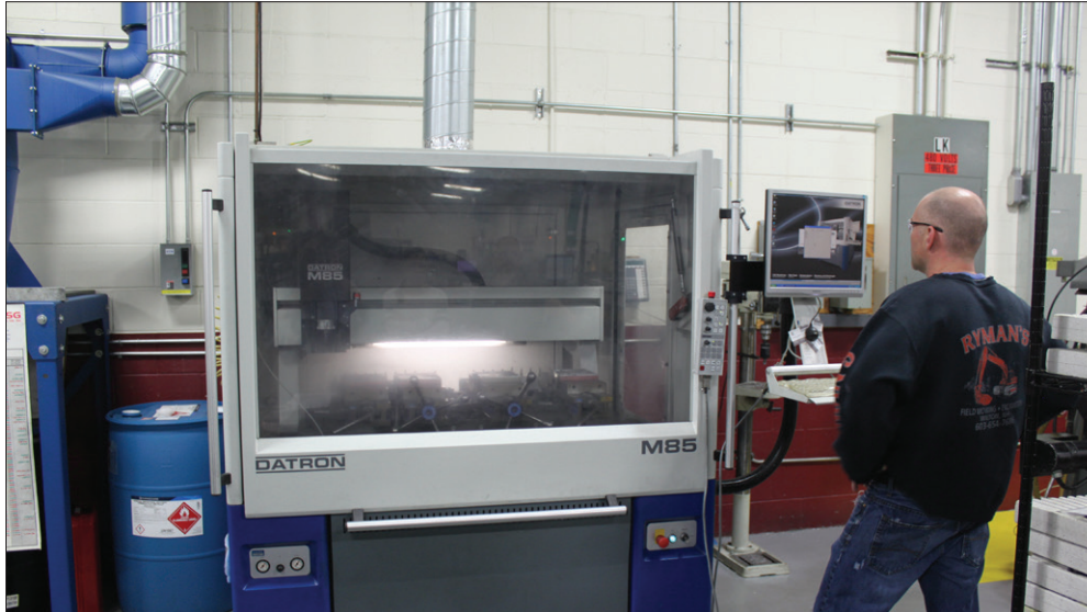
Haydon Kerk's DATRON machine operator initiates the milling program to run a batch of smaller rails.
