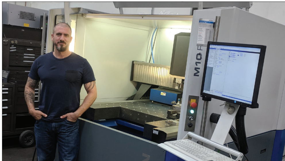
Hytech Tooling Manager, Dave Blandino with their DATRON M10Pro high-speed machining center.
