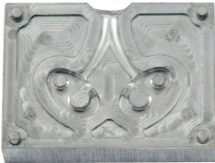
Bracelet clasp mold milled in aluminum on the DATRON neo.
