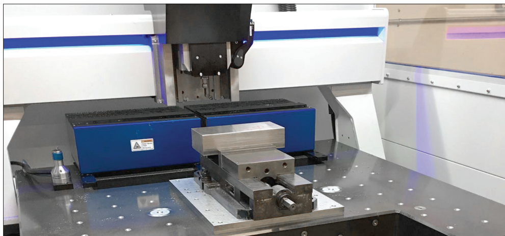
DATRON M8Cube's solid polymer-concrete bed setup for one of the many aerospace jobs that Rapid DTM runs in aluminum.
