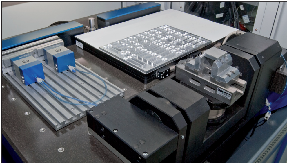
Multiple setups including pneumatic clamps, vacuum table and a trunnion rotary axis installed in the "cut out" of the bed.
