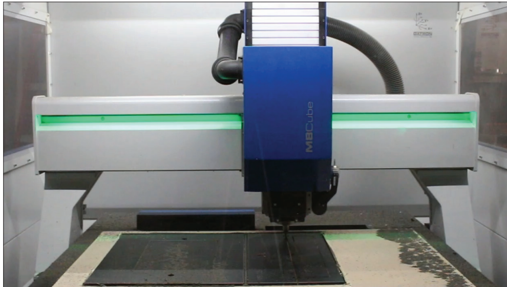
M8Cube's 40" x 32" work area provides ample room for sheet material to mill larger parts or nested milling of multiple parts.
